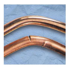
When an nVent ERICO brand of copper-bonded ground rod (top) and a copper-clad rod are subjected to the same pressure load, the inferior copper-clad rod (bottom) develops cracks and creases to the outer sheath. Damage to the rod negatively affects its serviceable life and puts the integrity of the entire electrode at risk.
