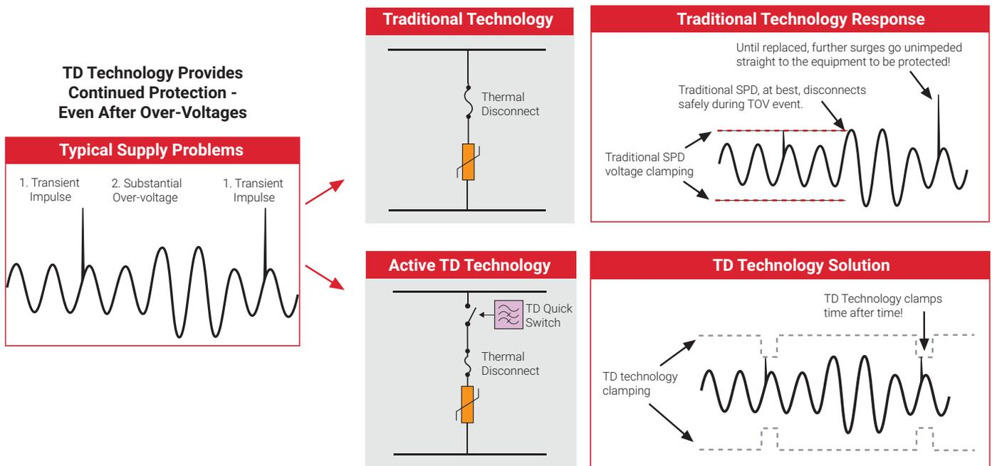
Effectively, TD Technology allows the SPD to have two clamping levels – one well above the peak of a TOV (up to twice its nominal AC voltage!), and the other much lower, to effectively and swiftly clamp lightning transients.
