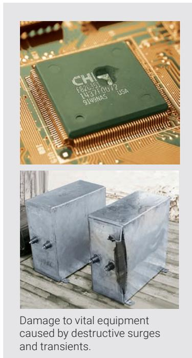
Damage to vital equipment caused by destructive surges and transients.
