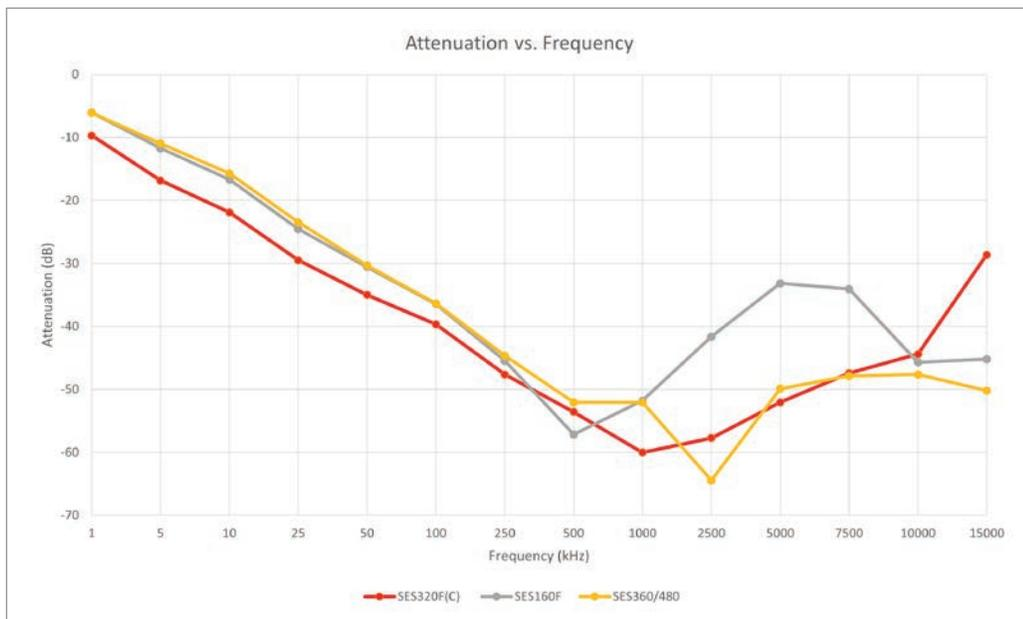
In this test (MIL-STD 220A), the filter is effective at reducing the amplitude of AC voltage signals, especially as a frequency of 500 kHz is approached. Attenuation across a range of frequencies appears to be consistent within the voltage range tested. Frequencies greater than 15 MHz resulted in the sinusoidal signal becoming distorted beyond recognition and the Vpp unable to be measured.
